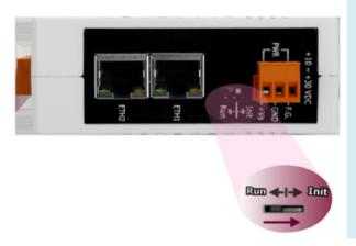
Step 2: Set the "Init Switch" to the "Init Mode" position.
