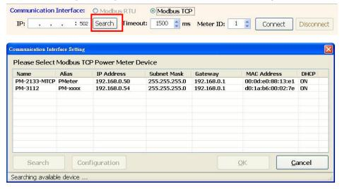
iv. Select the power meter which you want to modify parameters from the meter list, then click [Configuration] button to setup the meter parameters. After complete all setting, click [OK], and return to the meter list windows.
