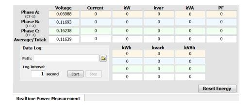
ii. When the power measurements have been read into the system, the Data Log function allows users to save the power measurements data into a file. Set up the file path and input the Log Interval (interval between each record), then click on "Start" button to perform the record of data.
