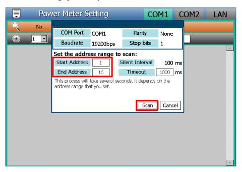
c. After the Scan operation is completed, a Modbus RTU power meter list will appear. After all settings are completed, click "Apply" button to save the changes.
