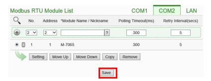
Please note: if fail to scan the I/O modules, please make sure the RS-485 cable is properly connected. And then go to Step 1: "System Setting"→"I/O Interface Setting" to make sure the settings of the COM Port that are connected to the I/O Module are accurate. After all settings are completed, click "Save" button to save the changes and repeat Step 3.a to perform scanning of the I/O modules again.
