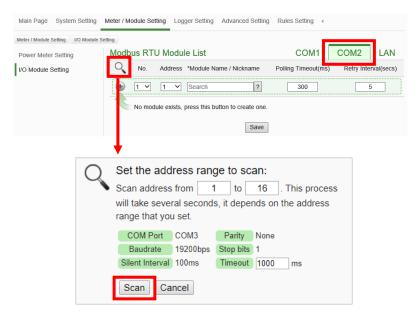
b. After the scanning is completed, the M-7000 I/O Modules connected to the COM Port interface will be displayed, click "Save" to complete the settings of the M-7000 I/O Module List.
