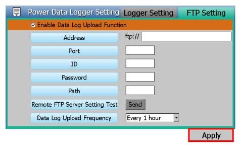
(5) Save the settings to PMD-420x, and then the Power Data Logger function will be enabled. The system will start to save the power data in the MicroSD card.
