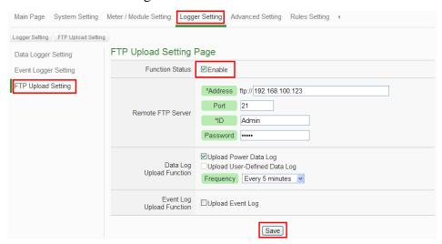
(3) Save the settings to PMD-420x, and then the Data Logger function will be enabled. The system will start to save the power data in the MicroSD card.
