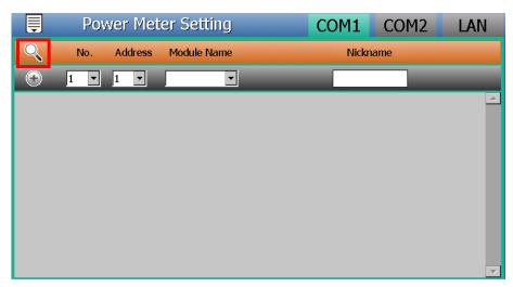
b. When the Scan page appears, input the starting address and the ending address of the Modbus address that are going to perform scan.
