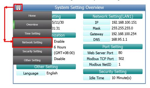
(3) Modify the PMD-420x network setting to fit current network environment.
