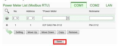
Please note: if failed to scan the power meters, please make sure the RS-485 cable is properly connected. And then go to Step 1: "System Setting"→"I/O Interface Setting" to make sure the settings of the COM Port that are connected to the power meter are accurate. After all settings are completed, click "Save" button to save the changes and repeat Step3.a to perform scanning of the power meters again.
