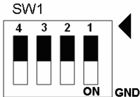
Fig. 1-10 SW1 setting for user controlled signals.
