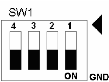
Fig. 3-13 SW1 setting for normally GND (Default setting)
