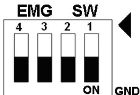
Fig. 3-13 EMG SW setting for normally GND (Default setting)
