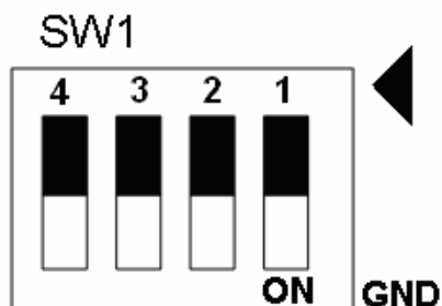
Fig. 3-14 SW1 setting for user controlled signals.
