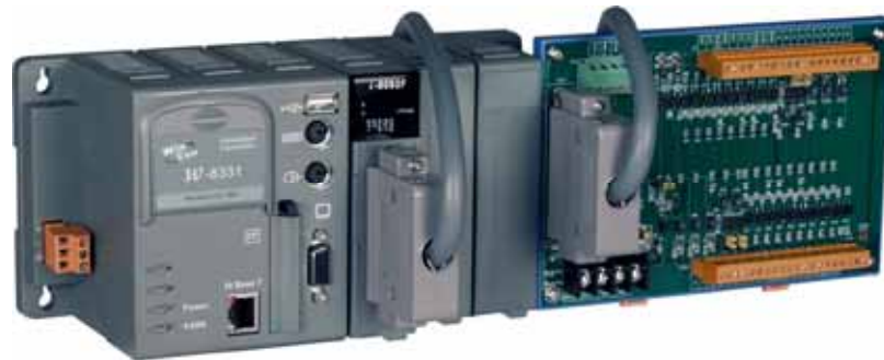
Figure. i8092F with PAC controller
