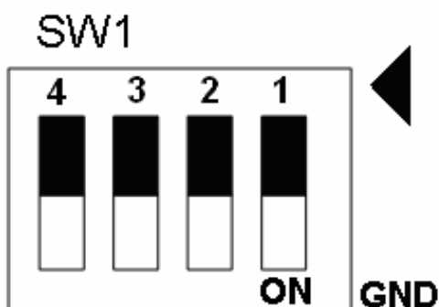
Fig. 1-10 SW1 setting for user controlled signals.
