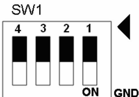
Fig. B3-9 SW1 setting for normally GND (Default setting)
