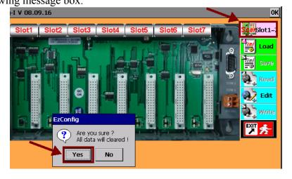
After a successful scan all the modules detected will be displayed with their names in their respective slots. In the background every IO channel of all the modules will be me mapped to an IO register number.
