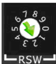
Fig.5 Shift rotary switch to 2
