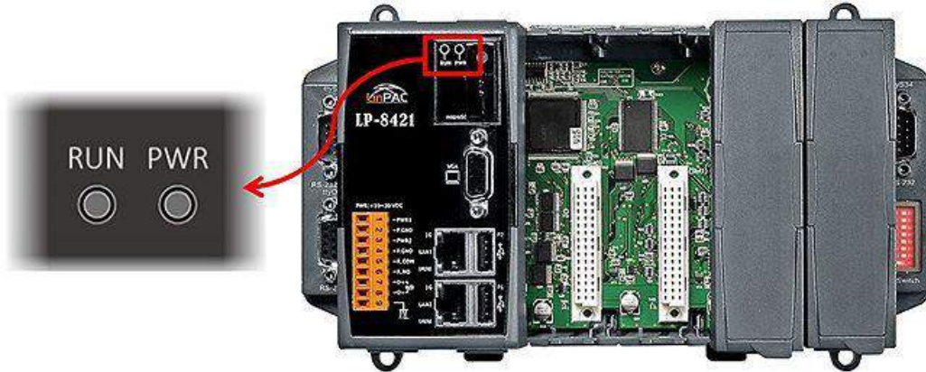
Figure 6.5.3-1. LED indicators for LP-8x2x series
