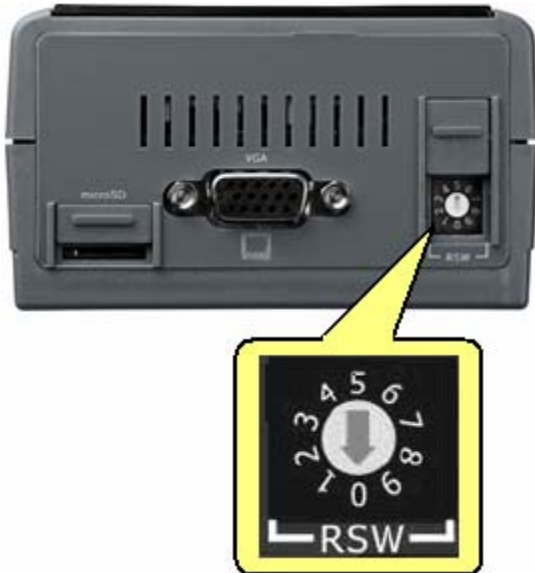
Fig. 15 Move the rotary switch to position 0
