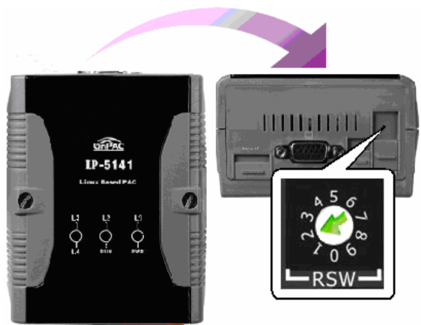
Fig. 11 Move the rotary switch to position 2
