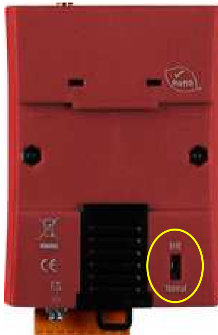
▲ Recovery to the factory configuration by Init switch
