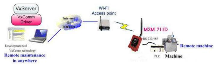
(2) Pair-Connection: This communication mode takes two M2M-711D modules, one works as an Ethernet Server; the other works as a Client, and use two computers to test and operate the M2M-711D modules. The architecture is shown below:
