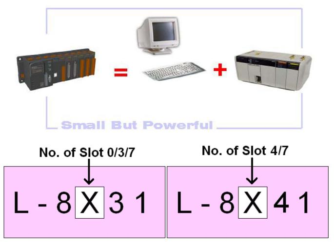
The LinCon-8x3x model type is ruled as L-8x31 and the LinCon-8x4x model type is ruled as L-8x41, as shown in the above figure. The Second number shows the slot numbers coming with the main controller unit. Currently, we provide three types of  $0 \cdot 3$  and 7 slots for LinCon-8x3x series and two types of 4 and 7 slots for LinCon-8x4x series. The last number demonstrates the application platform. 1 stands as the Master controller and it means that the user needs to design the
