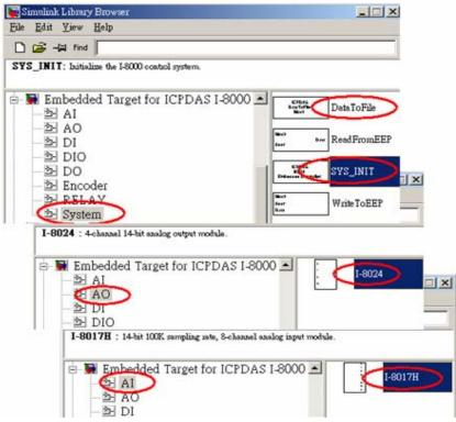
4.) Double-click on the I-8024 block, and then the dialog box appears. To use channel 0 of I-8024 module, enter [0] in the field "Output Channel". And select the slot as 2, Output Mode as "Voltage Out", Gain as 1 and Type of Value as "Floating".
