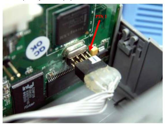
2. Power off WinCon-8000 and short B1 to B5 on any one of un-occupied slot connector in WinCon-8000. Power on again ,once WinCon-8000 detect B1 pin and B5 pin short together, boot-loader will search the OS image from the Ethernet port (instead of the flash memory) and issue a boot-me message.
