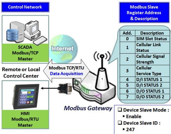
In addition to behave as a Modbus Gateway, there is an integrated Modbus Slave option for providing some device status, like Cellular Network Status, device DI/DO status, to remote Modbus Master via Modbus communication.
