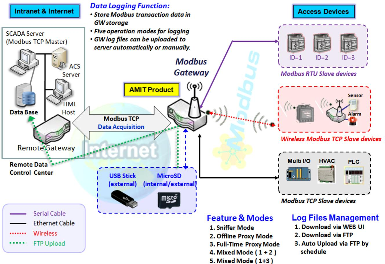
The Modbus Cellular Gateway provides a complete data logging function for collecting the Modbus transaction data for application requirements. There are some data logging schemes to meet different management requirements. They are the Sniffer Mode, Offline Proxy Mode, Full-Time Proxy Mode, and
