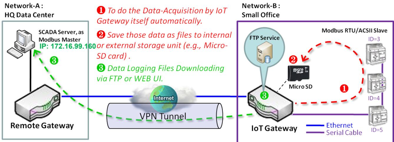
As illustrated, when the connection to a remote Modbus Master broken, the Modbus Gateway will activate the data logging proxy function and execute the pre-defined data acquisition task by itself.
