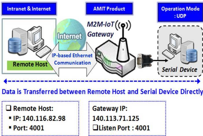
Data is Transferred between Remote Host and Serial Device Directly
