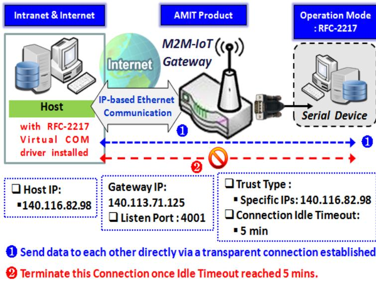
RFC-2217 defines general COM port control options based on telnet protocol. A host computer with RFC-2217 driver installed can monitor and manage the remote serial device attached to the gateway's serial port, as though they were connected to the local serial port. When a virtual serial port on the local serial device is being created, it is required to specify the IP-address of the host computers to establish connection with.
