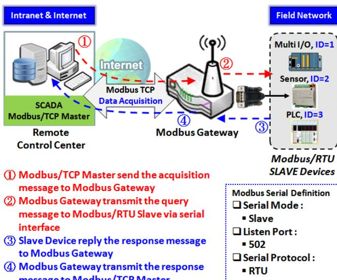
The IoT Gateway serves as a Modbus gateway to communicate with the Modbus TCP Master, the SCADA Server, located at remote control center for Modbus device accessing.
