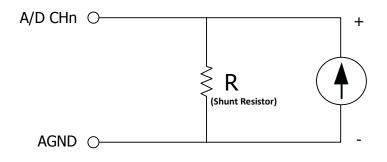
**Example:** A 20 mA source current through a 125  $\Omega$  resistor between + and – terminals and the board will read a 2.5 V<sub>DC</sub> voltage. You can use the **I** = **V/R** (Ohm's law) to calculate what value the source current should have.
