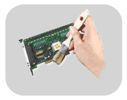
Note: Clean the board carefully when using soft brush.
