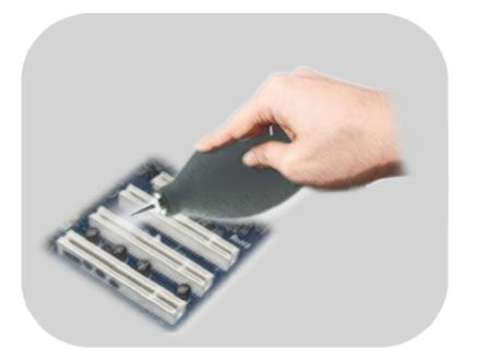
Step 6: Insert PCI/ISA/PEX card into the PCI/ISA/PCI Express slot carefully, and then power on the host PC.
