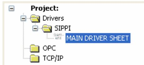
The MAIN DRIVER SHEET provides a simple way to associate Studio tags to addresses in the PLC. Most of the MAIN DRIVER SHEET entries are standard for any driver. Refer to the Studio *Technical Reference Manual* for information about the configuration of the standard fields. The fields that require specific syntax for this driver are described below:
