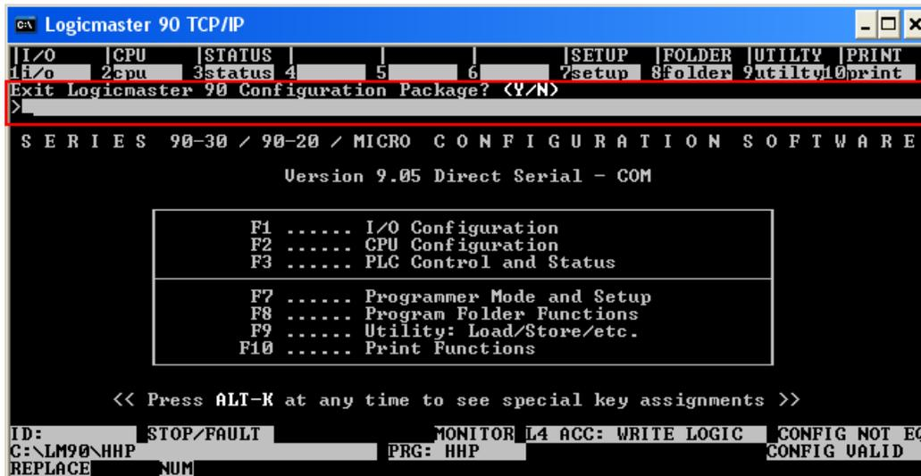
9. Confirm by pressing Y button. The main screen should be displayed (Figure 1).
