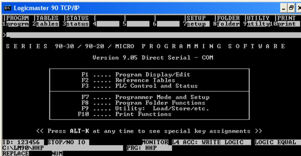
5. Select **Programmer Mode and Setup** by pressing F7 button. You should get the following screen, as follows below:
