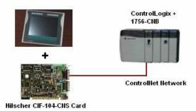
**2.2) DEVN:** This driver implements the **DeviceNet** slave using **Hilscher SMS-CIF104-DNS** PC card. This card has its firmware compiled also for WinCE and it has in the PC-104 format. So, in this case, you would need to install the Hilscher card CIF-104-DNS on your WinCE panel and this is will be a slave in the DeviceNet Network
