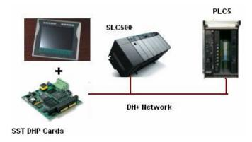
**3.2)STRIO:** This driver implements the AB **Remote I/O** protocol Scanner Mode to the family PLC5 using the **SST 5136-SD-104** card, implementing both the I/O and the Block Transfer
