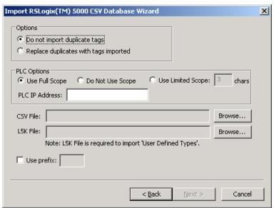
This interface allows the user to import the Tags Database and the communication interface configuration from the ControlLogix/FlexLogix PLC program files, including Allen-Bradley RSLogix CSV files. Before using this interface, you must export the project configuration using RSLogix 5000 programming software:
