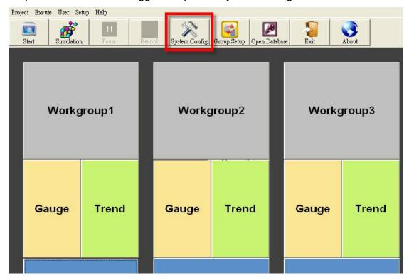
Step2. Input the connection setting  $\rightarrow$  tick "Log SQL Server"  $\rightarrow$  press "Save" button to save settings  $\rightarrow$  press "Exit" to leave the "System Config" form.
