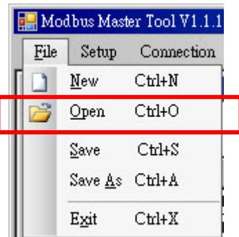
Step2. Select Module Series and Module List, and enter the slave ID (default is 1), and then click [Open]. If there is no module that want to be opened, go to step1 and select [New] to create a new configuration file.
