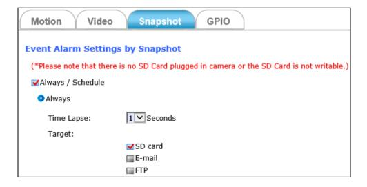
■ Schedule: This method activates the Camera snapshot operation continuously when the defined days of the week and set time of the set days are met.
