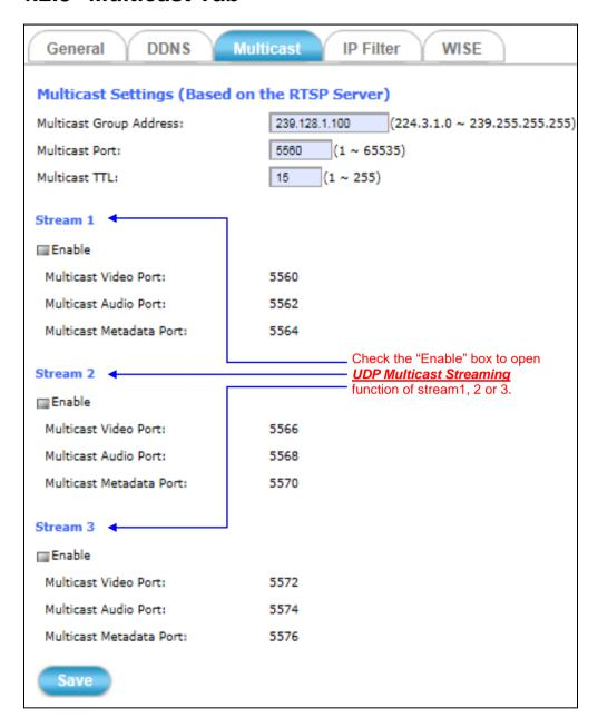
The **Multicast** tabbed pane allows you to open Camera's UDP Multicast Streaming function.
