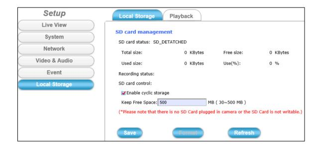
If recording is in progress when clicking the **Local Storage** button, a warning message will occur.
