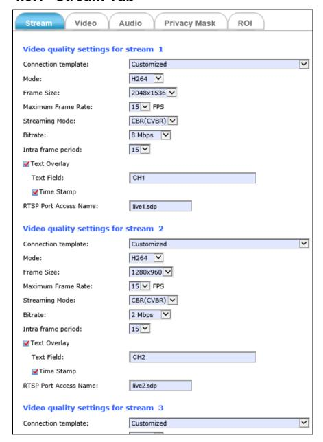
The **Stream** tabbed pane (see above figure) provides the adjustments for the video quality of the Camera streaming function.
