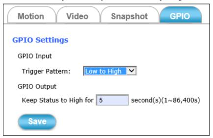
**GPIO Input:** To decide which kind of pattern would trigger event successfully. Options: Low to High, High to Low, or State Change.
