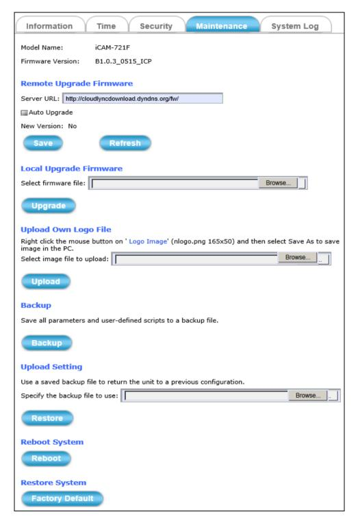
The **Maintenance** tabbed pane allows you to upgrade the firmware with the latest version and to restore the Network Camera settings to factory default.
