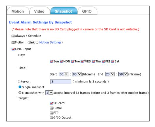
The stream of accumulated snapshots may be sent to host through E-mail, FTP, stored in the SD card, Remote Disk, activated GPIO Output Port; per selection or through all of them. When selected, the setup dialog for these methods will display is illustrated in the following figure.
