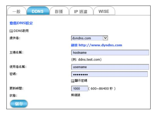
The **DDNS** tabbed pane allows you to configure the Dynamic Domain Name System of your network device with a host name instead of the IP Address.
