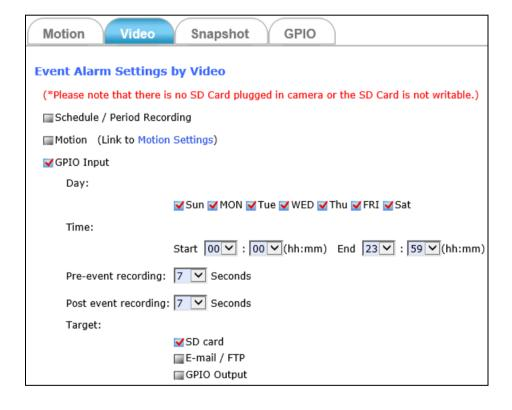
If selects the E-mail/FTP as the target, the user has to set up and test the E-mail Settings or the FTP Settings in the following figure.
