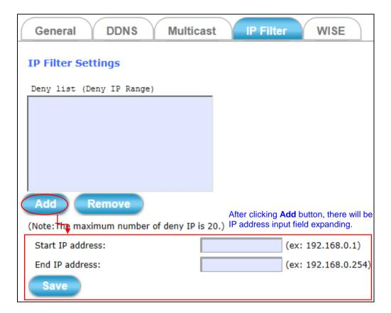
The **IP Filter** tabbed pane could let you configure device IP list which is denied access to this camera.
