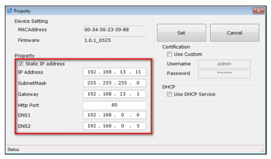
4. After modifying the camera properties, click [Set] button to save and enable the configuration modifications.
