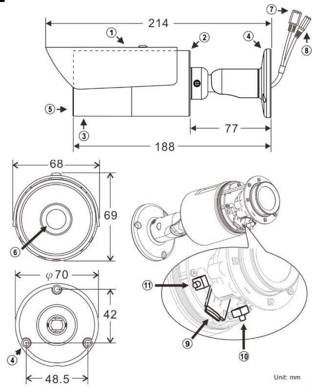
①Sun Shield ②Main Body ③Front Cover ④Bracket Base ⑤Window ⑥Lens ⑦RJ-45 Network Port (PoE supported) ⑧Power jack (DC12V ±10%) ⑨Micro SD card slot ⑩Factory default button ⑪Auto Focus button
