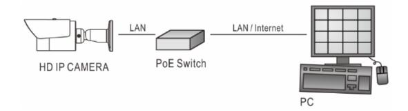
(3). Use PoE power injector and network switch connected to the network.
