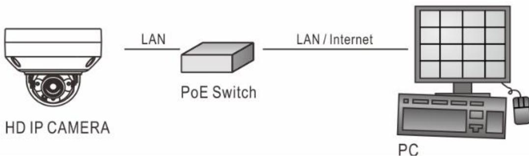
(3). Use PoE power injector and network switch connected to the network.
