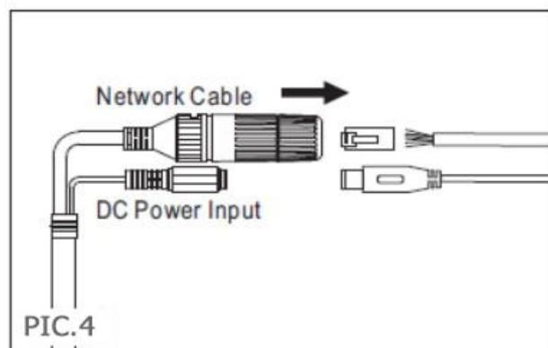
● *Connect the RJ-45 Ethernet cable with a waterproof connector*
