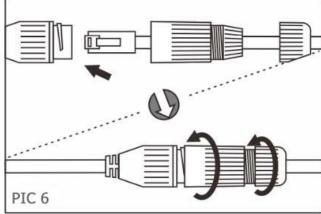
First, remove the waterproof connector and unscrew the waterproof nut. Insert the Ethernet cable and connect to the RJ-45 connector with proper tools (PIC.5). Then, tighten the waterproof connector and nut before the RJ-45 connector is connected to the camera (PIC.6).
