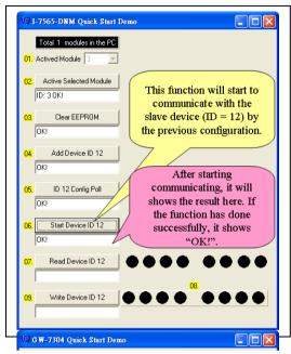
12. In this step, users can press these 8 LED button to edit the output data. And send the data to the output channel of the slave device (ID = 12) by pressing "Write Device ID 12" button to send the output data to the output channel of the slave device (ID = 12). At the same time, the D/O LED on I-8077 will show the same value.
