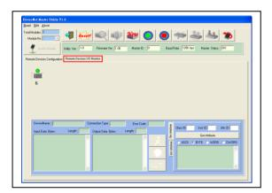
9. Pressing the icon picture to display the device information, including the device name and input data.
