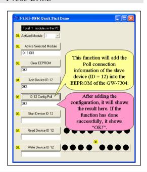
11. In this step, users can press the "Read Device ID 12" button to read the input data of the slave device (ID = 12). The input data is from the I-8077's 8 dip-switches. After changing the dip-switches, users can press the button again to refresh the LED status.
