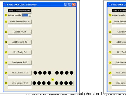
I-7565-DNM Quick Start Demo Total 1 modules in the PC When starting the demo Actived Module 3 program, it will search Active Selected Module how many I-7565-DNM module in the PC automatically. Clear EEPROM Add Device ID 12 ID 12 Config Poll Start Device ID 12 Read Device ID 12 Write Device ID 12
