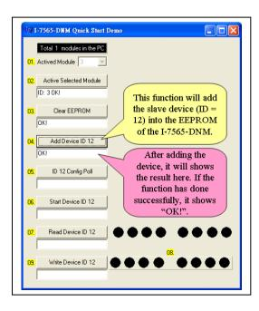
9. In this step, the user can press the "ID 12 Config Poll" button to add the Poll connection information of the slave device (ID = 12) into the EEPROM of the I-7565-DNM.
