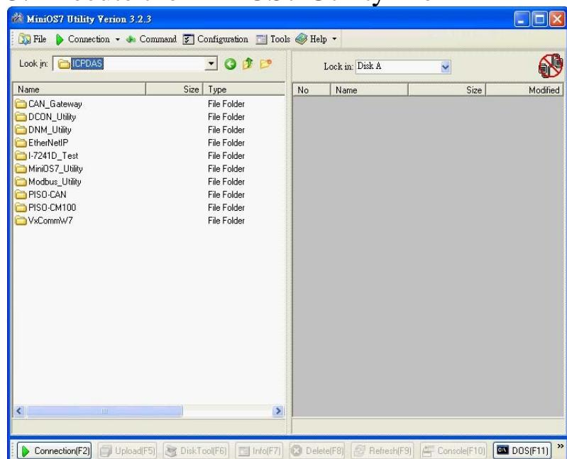
4. Press “Connection” button and select a necessary COM Port. Then Press “OK” button to start to connect with the I-7241D module.
