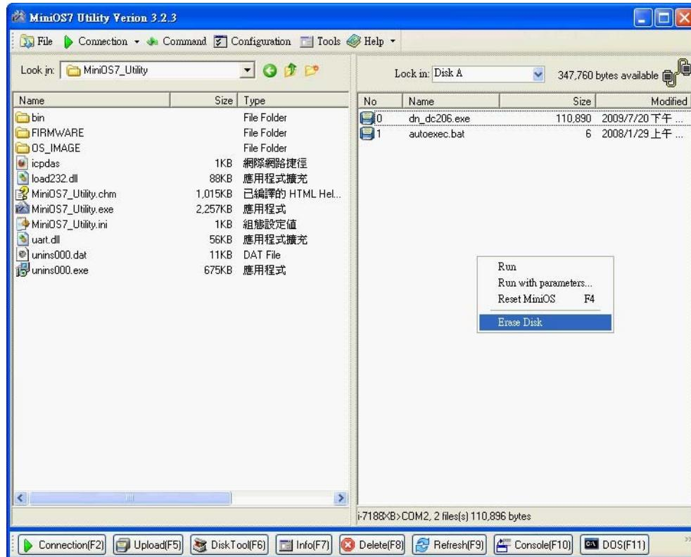
7. Select the “autoexec.bat” and “DN\_DC.exe” file. Right-click the mouse button and select “Upload” item to start to upload data into I-7241D’s flash.
