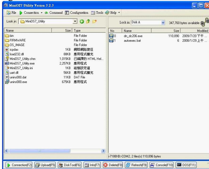
6. Right-click the mouse button on the right frame, and select “Erase Disk” item to erase all the data on the flash disk.
