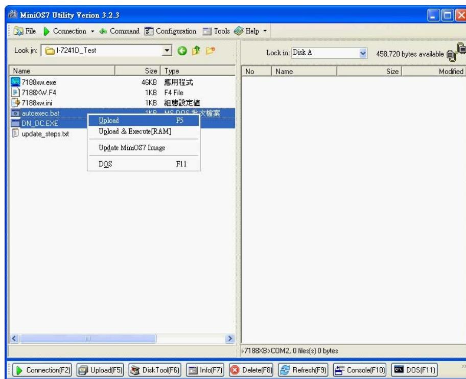
8. After uploading the firmware, please remove the line between INIT\* pin and GND pin, then reboot the I-7241D
