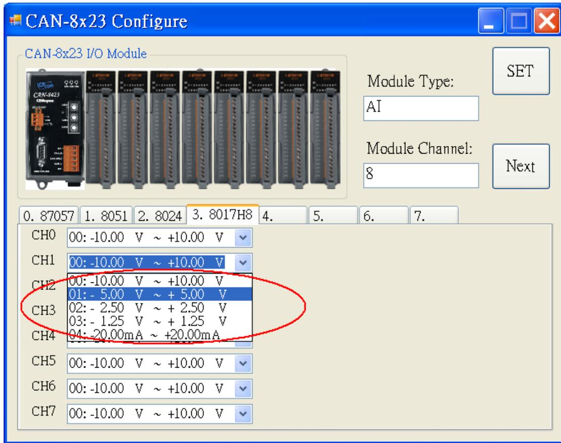
**Step 6:** After setting the proper output range, users can click “Set” button to store the configuration. If all of slot module configurations are finished, click “Next” button to next step
