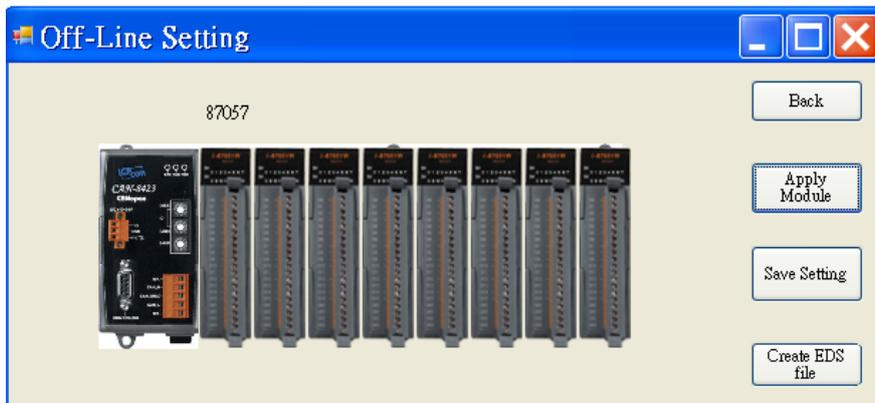
**Step 5:** Then, repeat the step 3~4 to configure the slot 1 to I-8042 module. Then, click “Save Setting” button to finish the off-line parameter settings..
