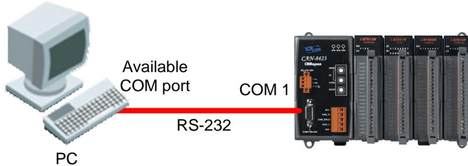
**Step 1:** Turn off the CAN-8423. Set the “Baud” rotary switch of CAN-8423 to 9 for configuration mode. Then Turn on the CAN-8423.
