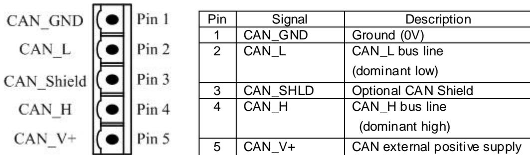
**CAN-8423 CAN bus connectors ping assignment**
