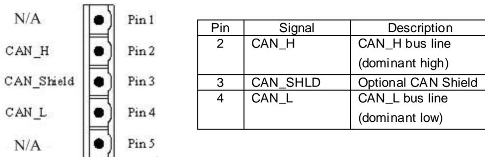
**CAN-8823 CAN bus connectors ping assignment**
