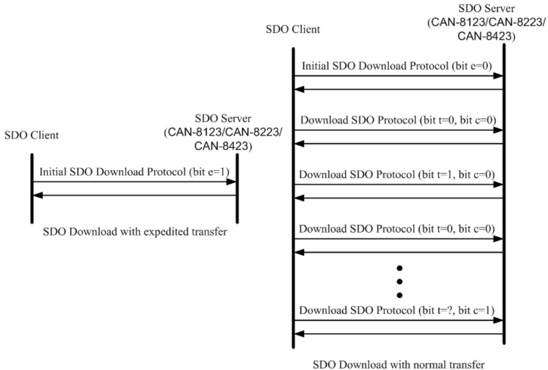
Since all of those object entries, which can be written, in the CAN-8123/CAN-8223/CAN-8423 are equal or less than 4 bytes, we can only provide the example for expedited transfer.
