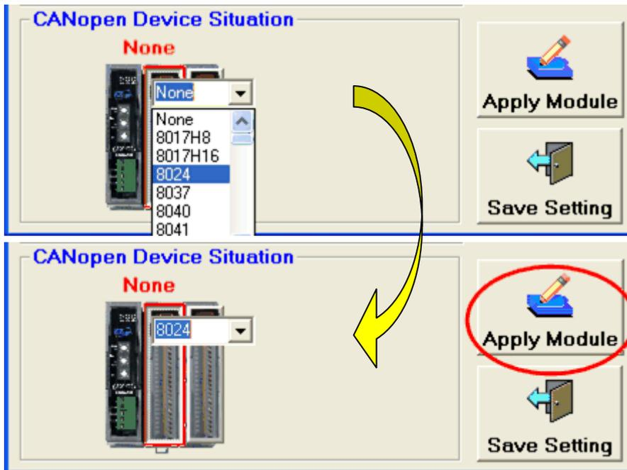
Step 4: After finishing the configuration, users can one-left click on the slot module in the “CAN Slave Device Situation” area. If the configuration is successful, users can see the correct module name, for example 8024 on the top of the slot module.
