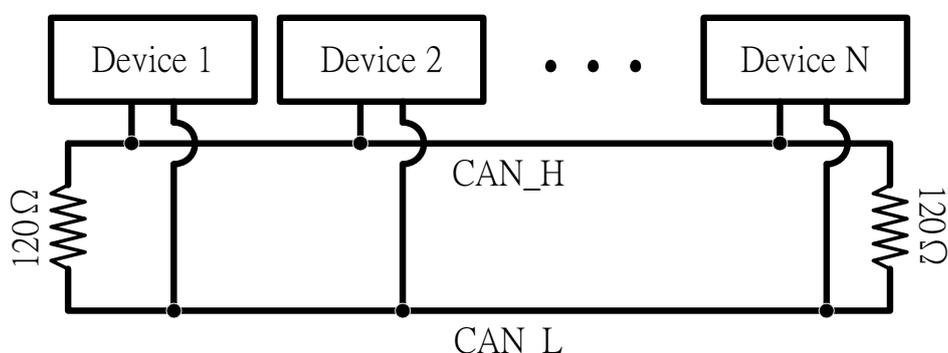
Moreover, to minimize the voltage drop, value of the terminal resistance must be higher than the one defined in the ISO 11898-2. The following table is for users' reference.
