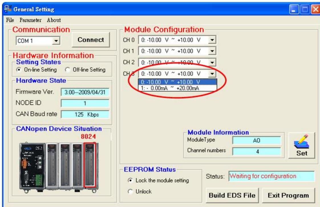
Step 6: After setting the proper output range, users can click “Set” button to store the configuration. If all of slot module configurations are finished, select “Lock the module setting” and click “Build EDS File” button to next step.
