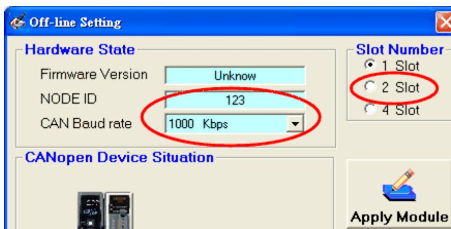
Step 3: Then, select a specific device presented in the “CAN Slave Device Situation” area, and choose a correct slot module inserted.
