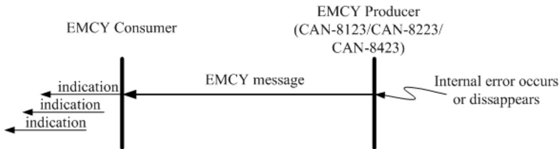
An emergency message containing 8-byte of data is called emergency object data. The abbreviated diagram is shown below, and all fields in the emergency object data will be described in section 5.3.
