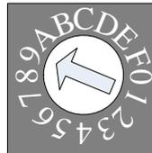
Step 2: Please use the “Baud” rotary switch again to set the baud rate for the CAN-8423, i.e. if users want to set baud rate in 1000Kbps, they have to adjust the “Baud” rotary switch to 7.
