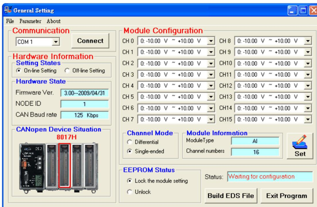
Step 5: Please select the slot module 4 in the “CANopen Slave Device Situation” area, and choose the output range in the “Module Configuration” area. Here, take the selection -10.00V~+10.00V as an example. Because of the feature of I-8024 slot module, output range on each channel will be
