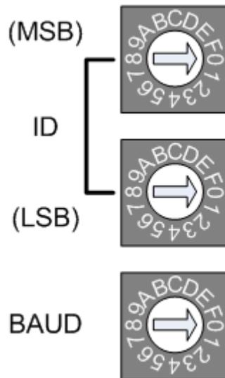
The first two rotary switches (MSB & LSB) control the CAN-8123/CAN-8223/ CAN-8423 node ID. MSB (Most Significant Bit) means the high nibble of the node ID, and LSB (Least Significant Bit). The last rotary switch (BAUD) handles the CAN-8123/CAN-8223/CAN-8423 baud rate. The relationship between the rotary switch value and the practical baud rate is presented in the following table.
