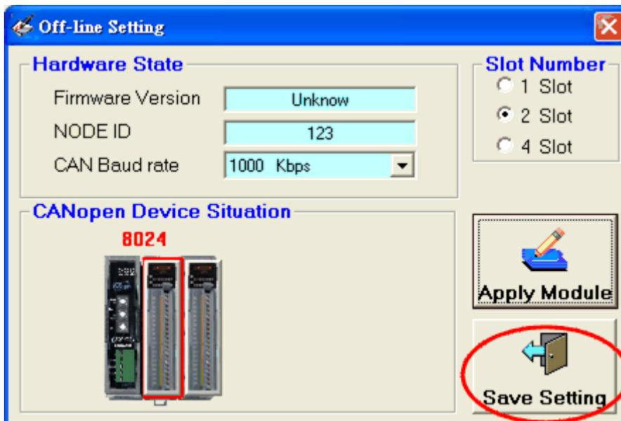
Step 5: Then, repeat the step 3~4 to configure the slot 1 to I-8042 module. Then, click “Save Setting” button to finish the off-line parameter settings.
