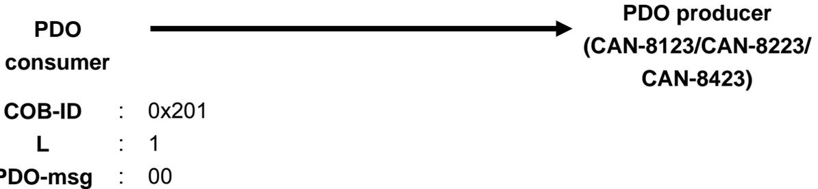
Step 2. Then, the CAN-8423 will reply to an emergency message based on the PDO data length of TxPDO1 doesn't correspond to the value defined in the PDO mapping object.
