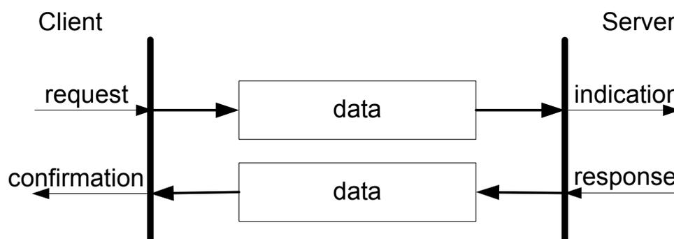
The SDO has two kinds of the COB-IDs, RxSDOs and TxSDOs. They can be viewed in the CANopen device. For example, users send a SDO message to the CAN-8123/CAN-8223/CAN-8423 by using RxSDO. On the contrary, the devices CAN-8123/CAN-8223/CAN-8423 transmit a SDO message by using TxSDOS.
