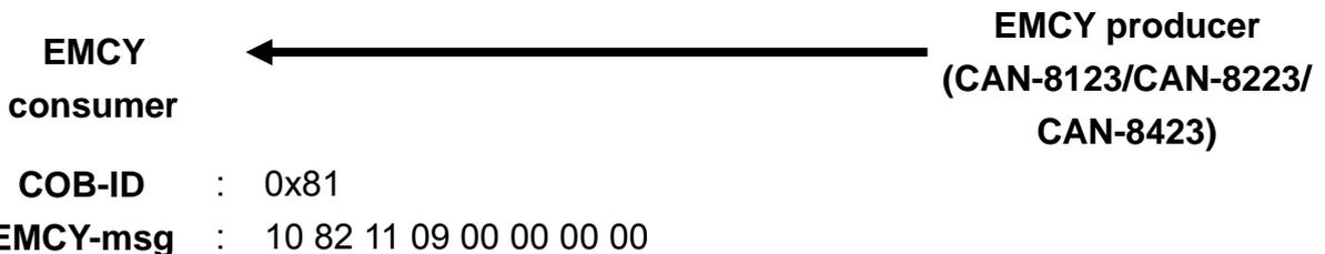
The first two bytes "10 82" are for the emergency error codes. The 3rd byte "11" is for the error register, i.e. the CAN-8423 has either a communication or a generic error. The last five bytes "09 00 00 00 00" are for the manufacturer specific errors. This emergency message means that the data length of TxPDO doesn't correspond to the value defined in the PDO mapping object.
