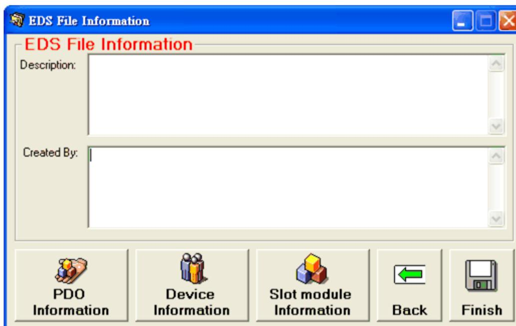
Step 8: Users can select the “PDO Information”, the “Device Information “and the “Slot Module Information” button for purpose to view the PDO objects, device profile and slot module configuration information. These information dialogs are shown below.
