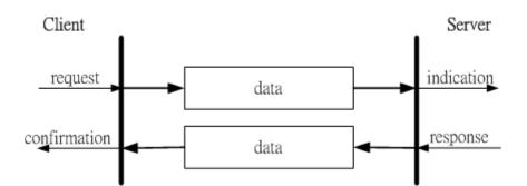
The SDO has two kinds of the COB-IDs, RxSDOs and TxSDOs. They are viewed at point in the CANopen device. For example, form the view of the I-7231D, if users want to send a SDO message, then the I-7231D needs to receive the SDO message transmitted from users. Hence, the receive SDO (RxSDO) COB-ID of the I-7231D will be used.
