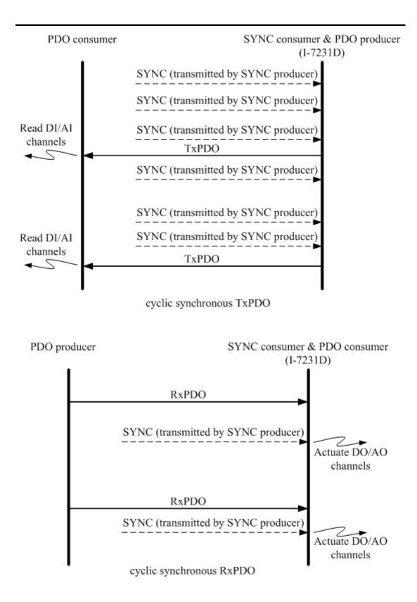
The RTR-only synchronous mode is activated when receiving a remote-transmit-request message and SYNC objects. This transmission type is only useful for TxPDO. In this situation, the I-7231D will update the DI/AI value when receiving the SYNC object. And, if the RTR object is received, the
