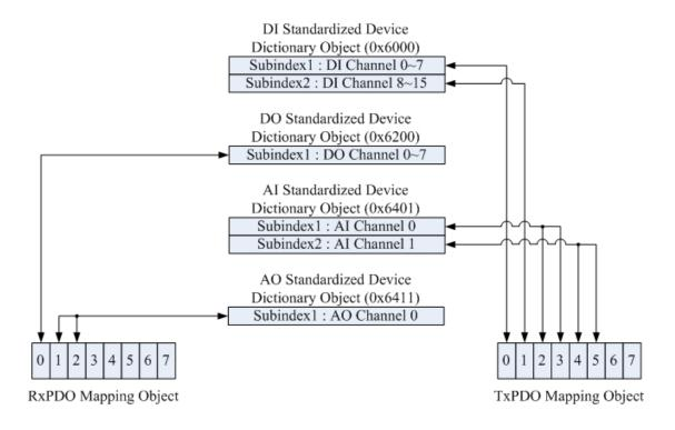
According to the PDO mapping objects in the figure above, if this CANopen device gets the RxPDO message including three bytes, the first byte is interpreted as the output value of the DO channels 0~7 and the following two bytes are the analog output value.
