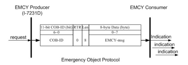
**COB-ID** : the EMCY COB-ID The EMCY COB-ID can be defined by user. This situation is similar to the PDO COB-ID. The default value is 4-bit function code "0001" with 7-bit node ID.
