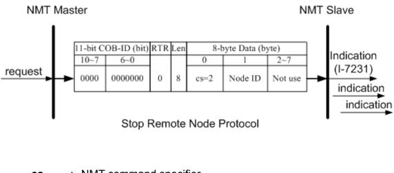
cs : NMT command specifier 2: stop Node ID : the node ID of the NMT slave device
