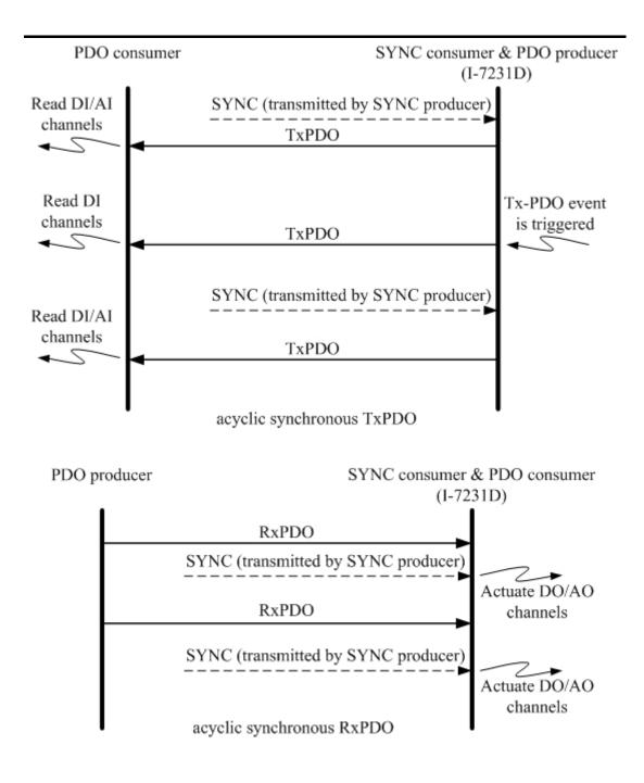
The cyclic synchronous transmission mode is triggered by the reception of an expected number of SYNC objects, and the max number of expected SYNC objects can be 240. For example, if the TxPDO is set to react when receiving 3 SYNC objects, the I-7231D will feedback the TxPDO object after receiving 3 SYNC object. For the RxPDO, actuating the DO/AO channels by the RxPDO is independent of the number of SYNC objects. These concepts are shown in the figures below.
