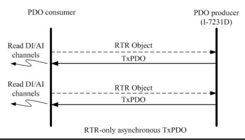
The other part of the asynchronous mode is the asynchronous transmission type. Under this transmission type, the TxPDO message can be triggered not only by receiving the RTR object but also by the occurrence of TxPDO events described in the event driver paragraph described above. Furthermore, the DO/AO channels can act directly by receiving the RxPDO object. This transmission type is the default value when the I-7231D boots up. The concept of the asynchronous type is illustrated as follows.
