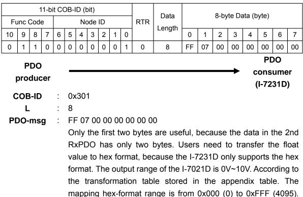
Therefore, the 5V is mapped to the 0x7FF by applying following equation.
