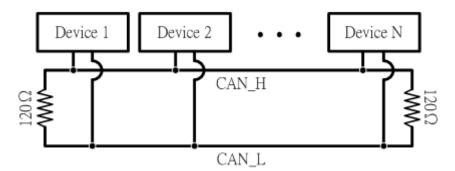
Moreover, to minimize the voltage drop on long distance, the terminal resistance should be higher than the value defined in the ISO 11898-2. The following table could be a reference.
