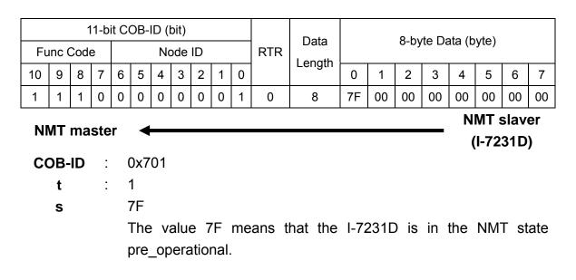
Step 6. Since life time is equal to 1000 ms (guard time \* life time factor =250\*4=1000), users will need to transmit the node guarding protocol again. If not, an error event will be triggered, and an EMCY message will be received. All values from the output channels will be changed according to index 0x6206, index 0x6207, index 0x6443, and index 0x6444.
