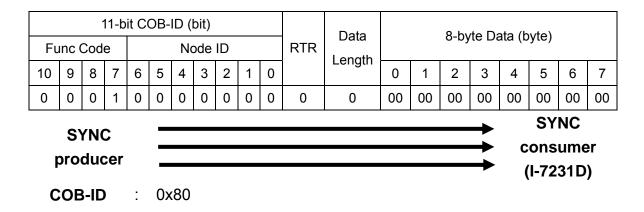
Step 26. After finishing the transmission of the three SYNC objects, the 1st TxPDO is triggered, and users can receive the 1st TxPDO from I-7231D.
