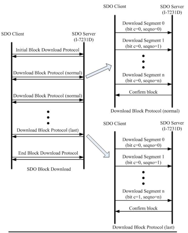
Step 1. In order to inform the I-7231D that the value of the object entry with index 0x1400 and sub-index 02 will be modified by using the SDO Block Download method, the Initiate SDO Block Download protocol is implemented.
