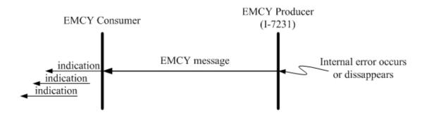
An emergency message contains 8-byte of data called emergency object data, and follows the structure provided bellow.
