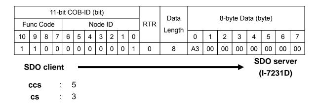
Step 4. The I-7231D responds to the first 7 bytes of data by using the Upload SDO Block Segment protocol.
