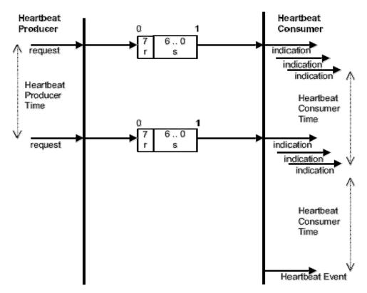
The Heartbeat Protocol defines an Error Control Service without need for remote frames. A Heartbeat Producer transmits a Heartbeat message cyclically. One or more Heartbeat Consumer receive the indication. The relationship between producer and consumer is configurable via the object dictionary. The Heartbeat Consumer guards the reception of the Heartbeat within the Heartbeat Consumer Time. If the Heartbeat is not received within the Heartbeat Consumer Time a Heartbeat Event will be generated.
