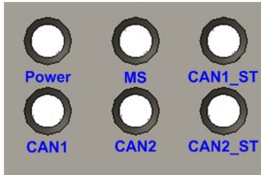
Figure 2-3 LED Assignment of I-7565M-HS
