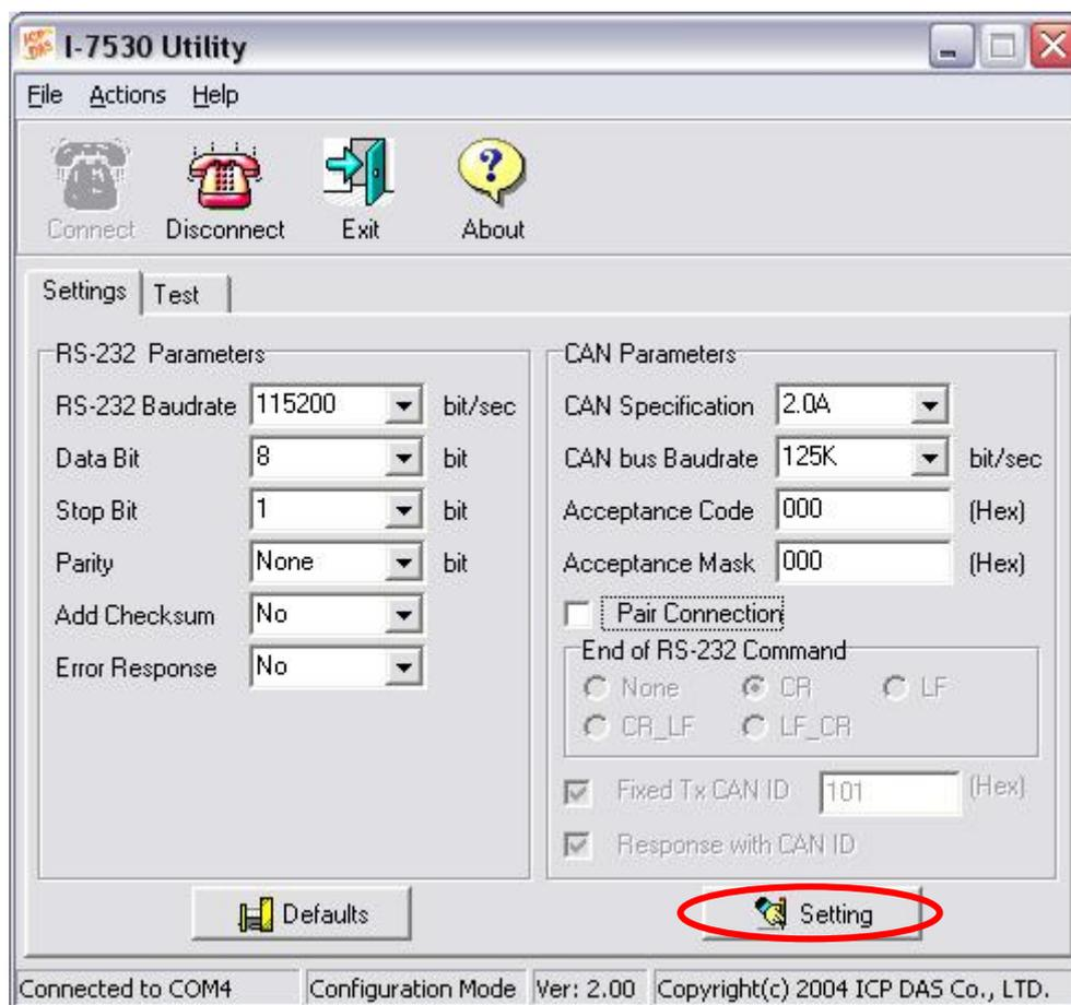
Step6: In order to match the RS-232 parameters on the PC COM port, please configure the RS-232 parameters of the I-7530A\_A as follows:
