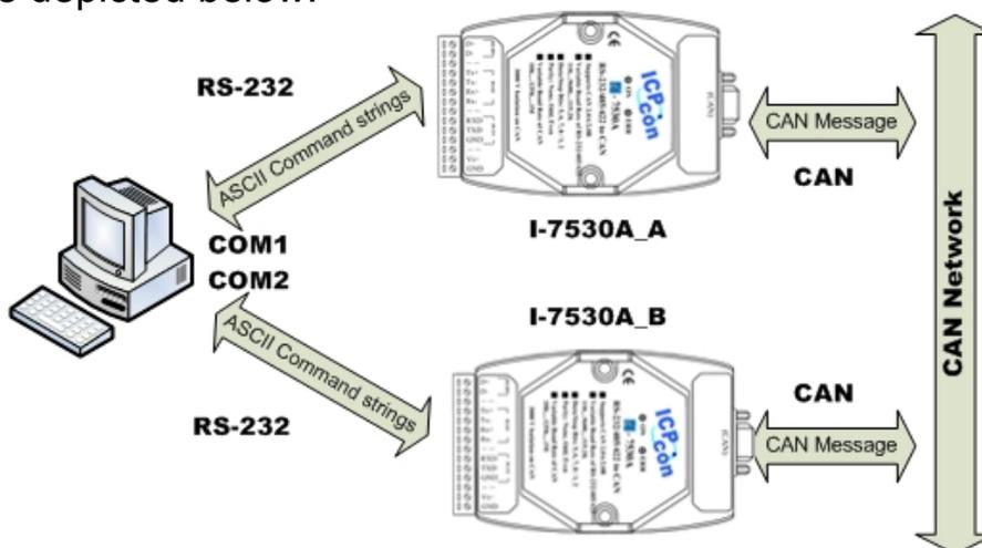
When the I-7530A receives a valid RS-232/485/422 message with the ASCII strings format, it converts this string into a CAN message and transmits it into the CAN network. Based on the same reasoning, when a CAN message is received via the I-7530A, the message will be
