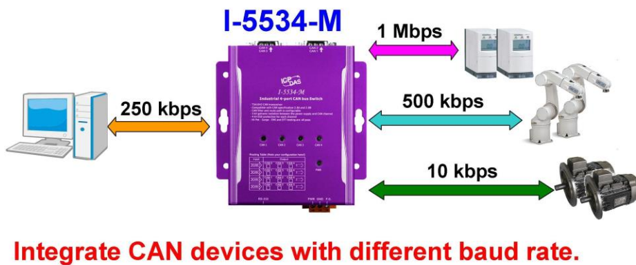
Figure1-2: Application to integrate the devices with the different baud rates.
