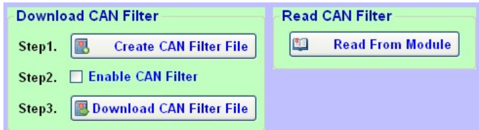
Figure 4-3 Set and read the CAN filter configuration
