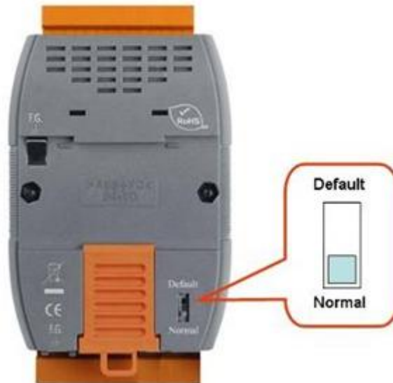
Figure 12-1: DIP Switch of the HRT-710
