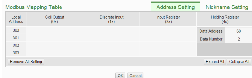
Figure7-50 : Input Register Setting Example for Modbus RTU Module
