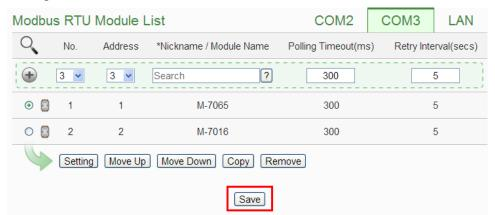
Please note: if fail to scan the I/O modules, please make sure the RS-485 cable is properly connected. And then go to <u>Step 1</u>: "System Setting"  $\rightarrow$  "I/O Interface Setting" to make sure the settings of the COM Port that are connected to the I/O Module are accurate. After all settings are completed, click "Save" button to save the changes and repeat <u>Step 3.1</u> to perform scanning of the I/O modules again.
