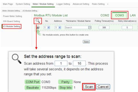
3.2 After the scanning is completed, the M-7000 Modules connected to the COM Port interface will be displayed, click "Save" to complete the settings of the M-7000 I/O Module List.
