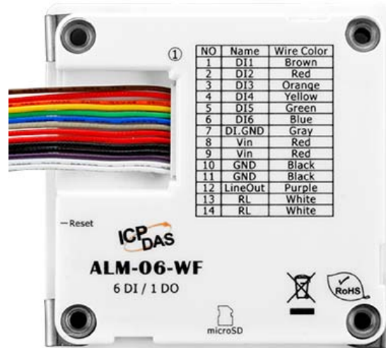
Figure 2-6: Wire color & function
