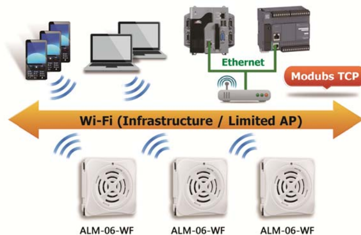
Figure 1-1: Application architecture for the ALM-06-WF
