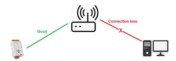
The Idle Timeout for Modbus TCP connection (default is **120 Sec**), user can change it from PC utility, Android APP, HTML or Modbus TCP Command. For more detail please reference to each User's Manual.
