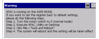
**Step 3: Turn** the rotary switch on the device to "0" and reboot.
