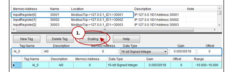
Click the **Scaling** button and choose a **Channel Type** (e.g., -10 to 10 V), and then click **OK**. Then, both the **Gain** and **Offset** values will automatically be set in the respective fields.
