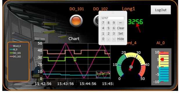
Note: To test negative value, first set the Long1 as a negative value on the local HMI page on PAC.
