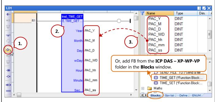
**Note:** All parameters of function block must be assigned a variable even if only the "PAC\_ss" variable is used in the project.
