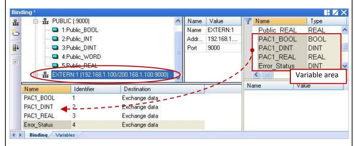
8. As the picture below, "Error\_Status" variable is used to determine the communication status of the PAC, please set this ID to "0" and then double-click "Destination" field and set it to "Connection error status".
