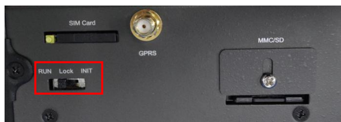
Figure 2-1 : The switch is located at the back of the controller
