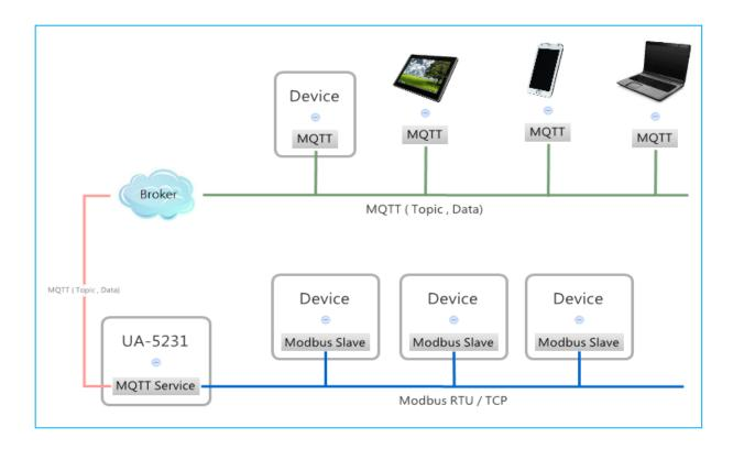
The following steps will show you the way to convert the Modbus Master Input's data into the MQTT message.
