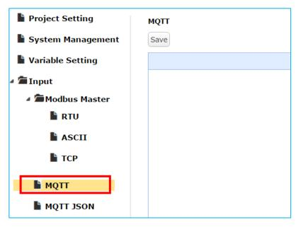
**Step 3**Add a MQTT Task. Set Task name and Broker information according to your project.
