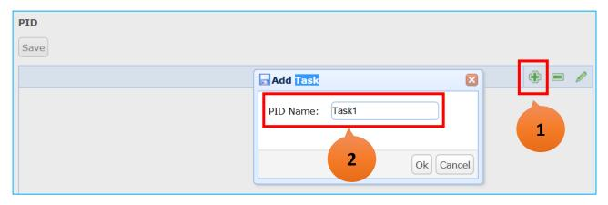
Set up the PID parameters. Assign an input variable to PV, an output variable to MV, and set other parameters according to the project needs. The user can set the "Auto Tune" as "true" for automatic PID regulator, but still has to enter some important parameters such as "Sample Time", "SetValue"... (See Section 3.5.1 PID for details).
