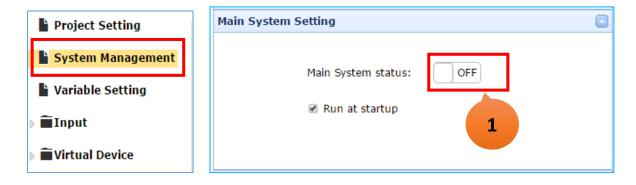
While "ON" is displayed, it means the new project is running in the UA-5200 system.
